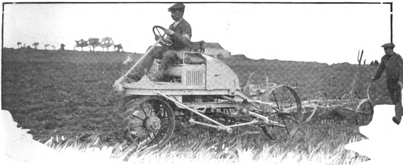
De Mesmay gasoline motor hoe worked at a cost of 74 cents per acre in the tests
